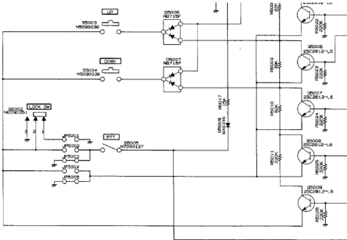
Fig 1 is a section of the schematic for the MH48 Microphone. The complete schematic is located in the files section... [thanks to who ever posted that schematic.](#)
