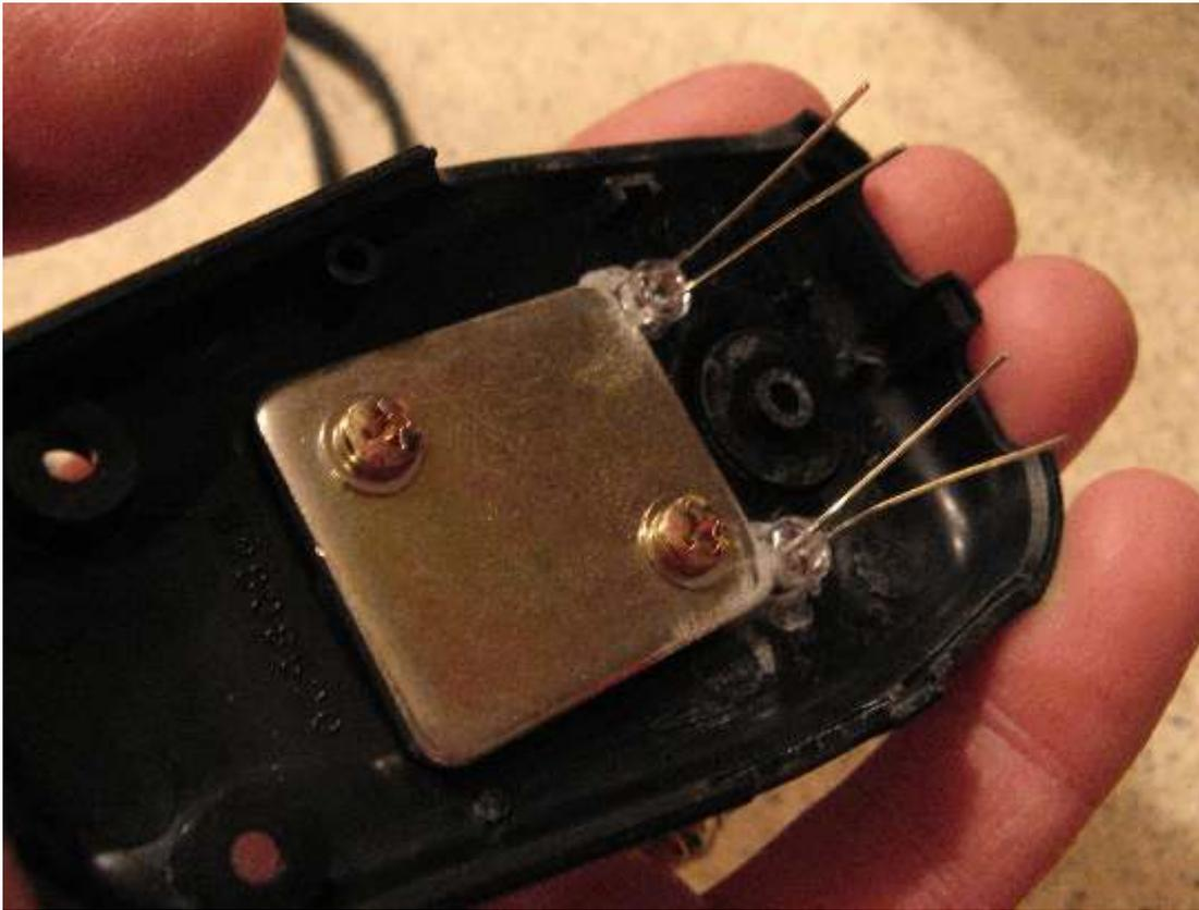
Be careful when locating the spot to drill for the LED holes... watch out for the metal "weight".
